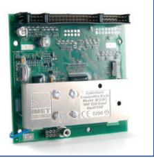
**The electronic boards are coated** with a special protective synthetic film for improving the resistance to humidity, chemical agents and vibrations.
